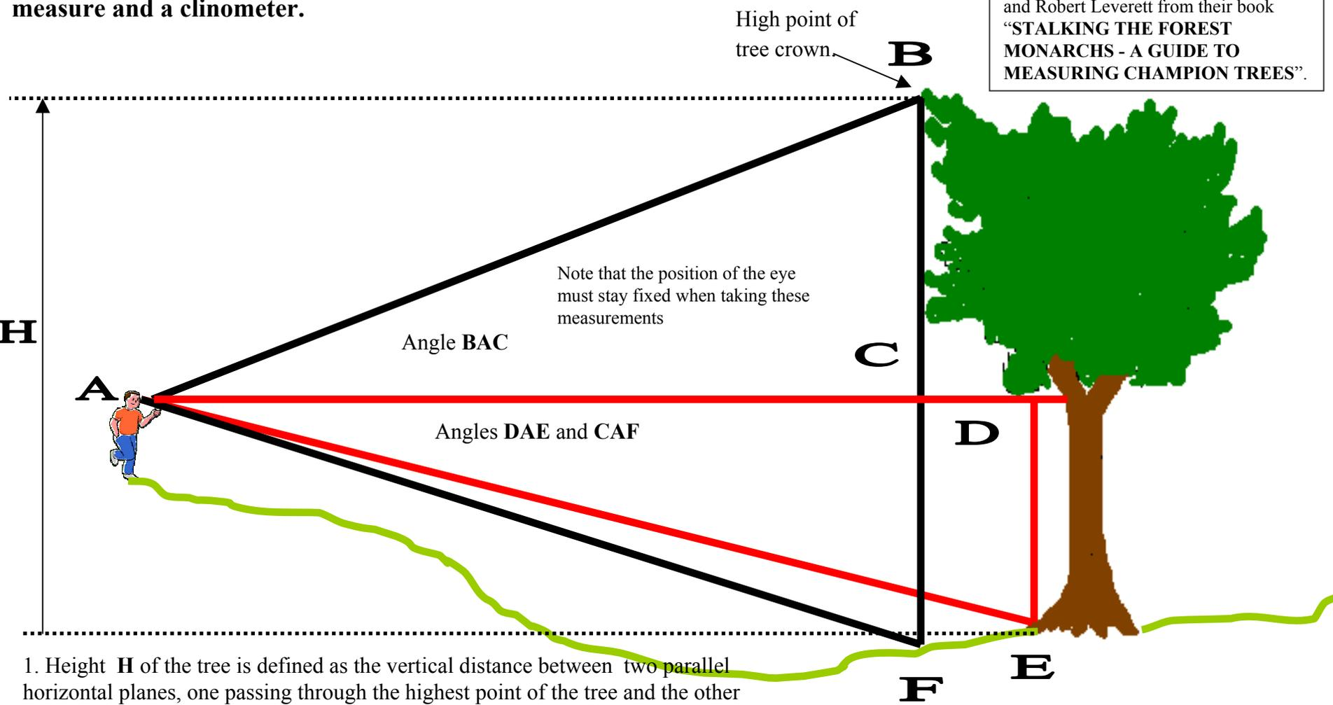
1. Height **H** of the tree is defined as the vertical distance between two parallel horizontal planes, one passing through the highest point of the tree and the other passing through the base of the tree. This height can be divided into two segments **BC**, the component above eye level, and **CF**, the component below. Note that height is not synonymous with tree length.
